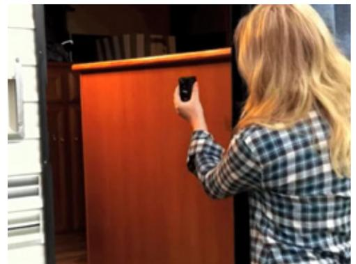
**Vertical surface:** Ensure front face of Transmitter is facing toward front of caravan.
